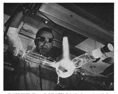
GLASSBLOWER Clinton Tuthill (4221-4) is shaping a quartz bulb using a large hydrogen/oxygen torch. His deep blue glasses filter out the intense light from the temperatures which approach 1700°C.
